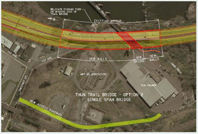
Figure 41: Option 2 – Single Span Replacement
