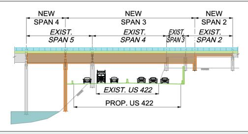
Figure 31: Option to Replace Only Impacted Spans on Rail Road Bridge
