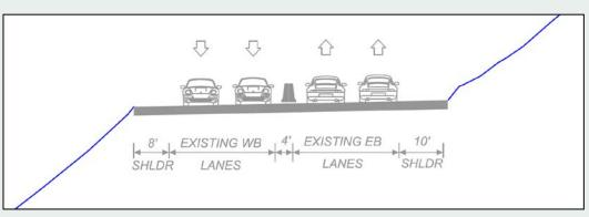
Figure 14: Typical Section of Existing Conditions Section 1 – East of Wyomissing Boulevard Interchange
