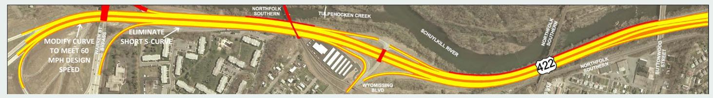
It was determined that there is 50 feet between piers if the road is realigned to be parallel to the piers. Even when the section could be realigned to be parallel to the piers, substandard shoulders will exist in the proposed condition.
