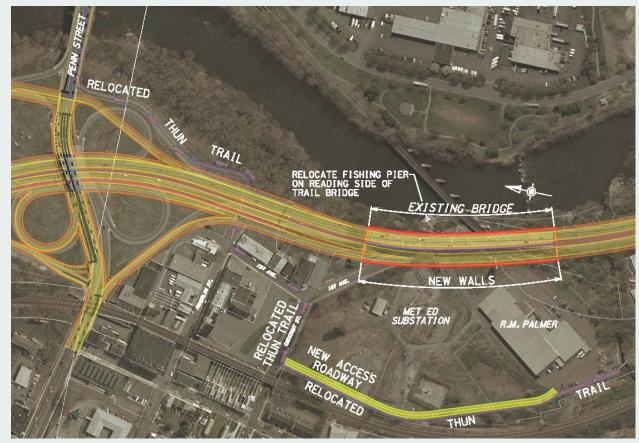
Figure 42: Option 3 – Eliminate Bridge
