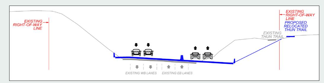
Figure 44: Proposed Roadway Crossing Showing Asymmetrical Widening
