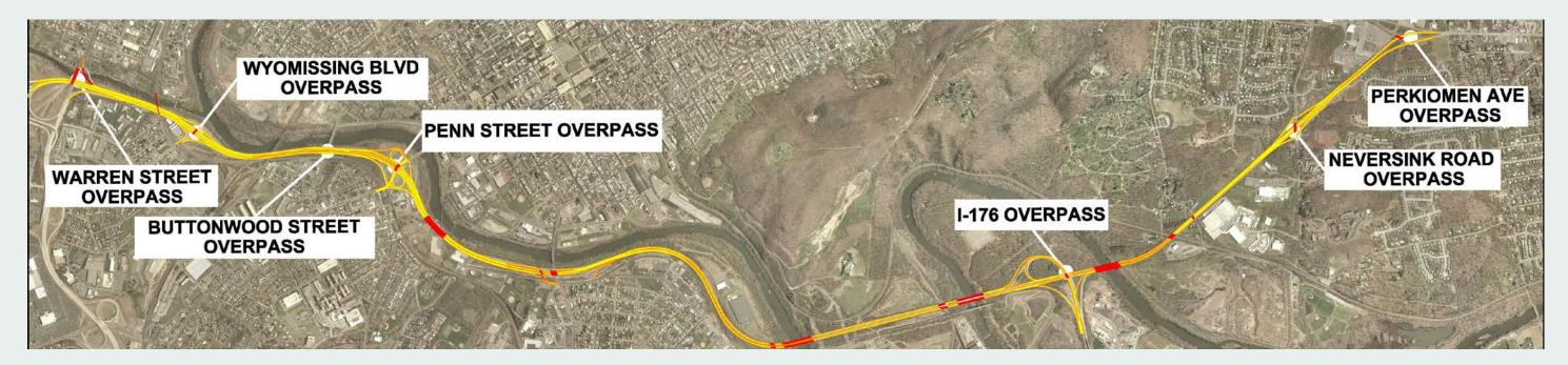
road, those ramps could be constructed first with temporary connections to existing US 422 eastbound. This approach would remove US 422 eastbound access from the left side, which is desirable. And since the westbound access ramps are proposed where existing US 422 westbound is located or go under the entire road, these ramps will need to be detoured during construction. This detour is discussed below.
