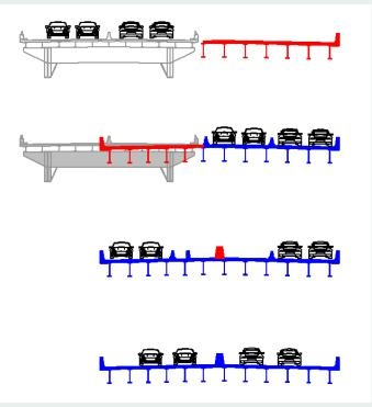
Figure 46: Reconstruction with Alignment Shift
