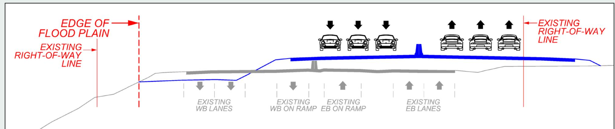
Figure 37: Proposed Roadway Cross Section Showing Avoidance of Floodplain Encroachment
