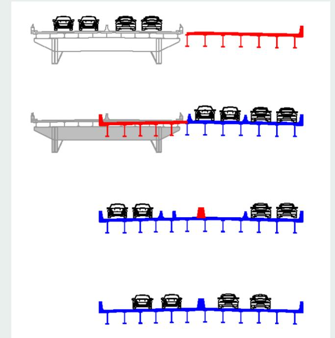
Figure 46: Reconstruction with Alignment Shift
