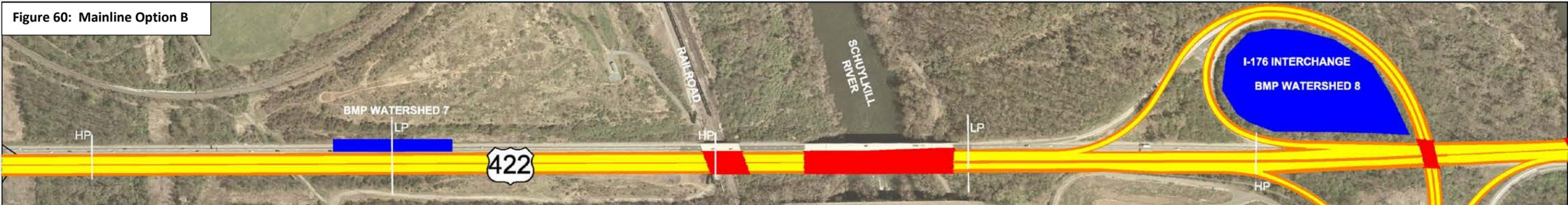
Watershed 7 is from the western end of Watershed 6 (HP approximately 620' east of the Schuylkill River crossing) to the HP over the railroad. The LP for this watershed is approximately 1330' west of the railroad crossing. The BMP for Watershed 7 could be located at this LP in the median of US 422 for Mainline Option A (**Figure 59**) and along the eastbound lanes of US 422 for Mainline Option B (**Figure 60**).
