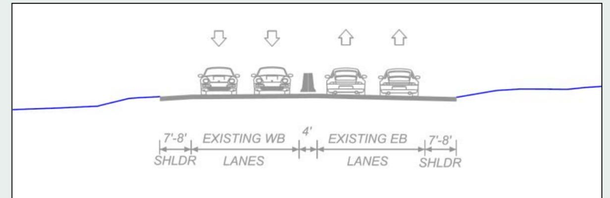
**Figure 24: Typical Section of Existing Conditions
