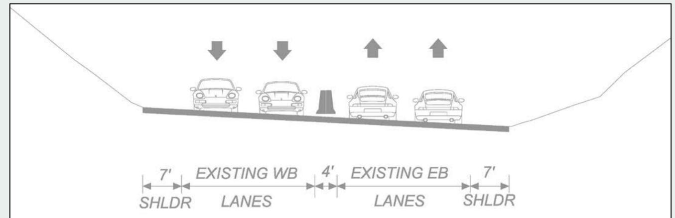
**Figure 21: Typical Section of Existing Conditions**
