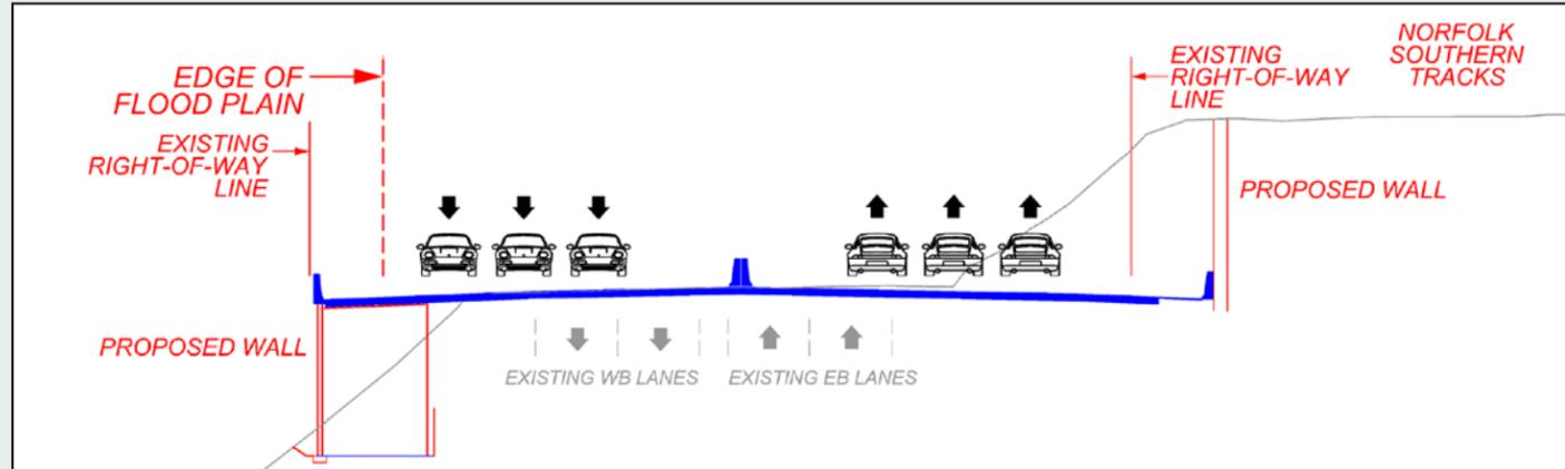
Figure 33: Proposed Roadway Cross Section Showing Floodplain Encroachment
