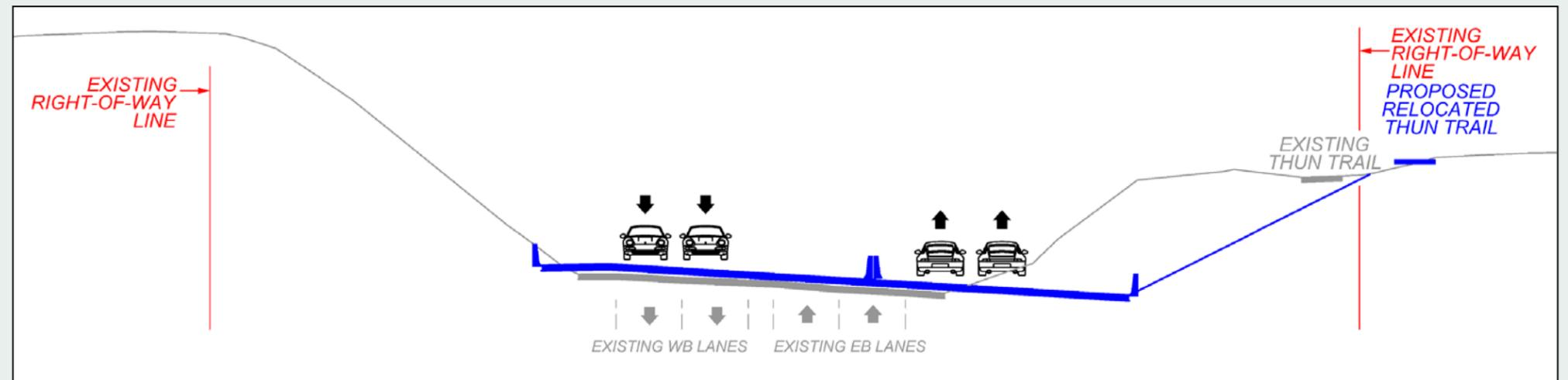
Figure 44: Proposed Roadway Crossing Showing Asymmetrical Widening
