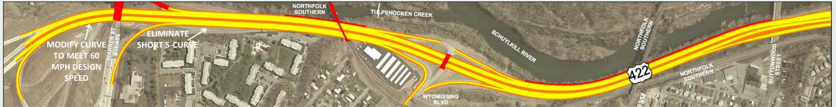
It was determined that there is 50 feet between piers if the road is realigned to be parallel to the piers. Even when the section could be realigned to be parallel to the piers, substandard shoulders will exist in the proposed condition.
