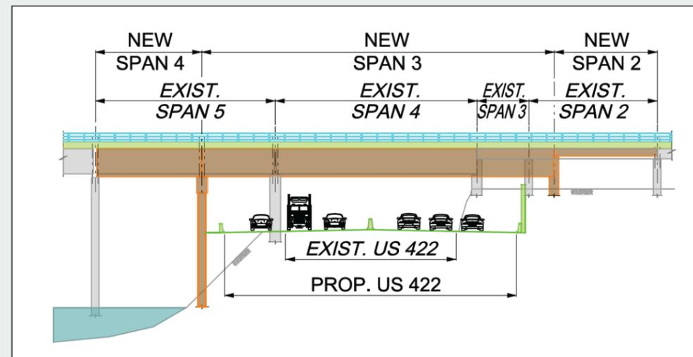
Figure 31: Option to Replace Only Impacted Spans on Rail Road Bridge
