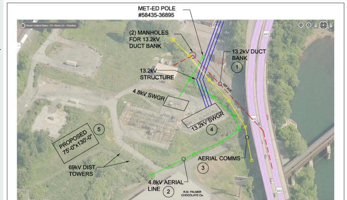
**Figure 63: Met-Ed West Reading Substation**
