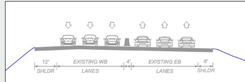
**Figure 13: Typical Section of Existing Conditions Section 1 – West of Wyomissing Boulevard Interchange**
