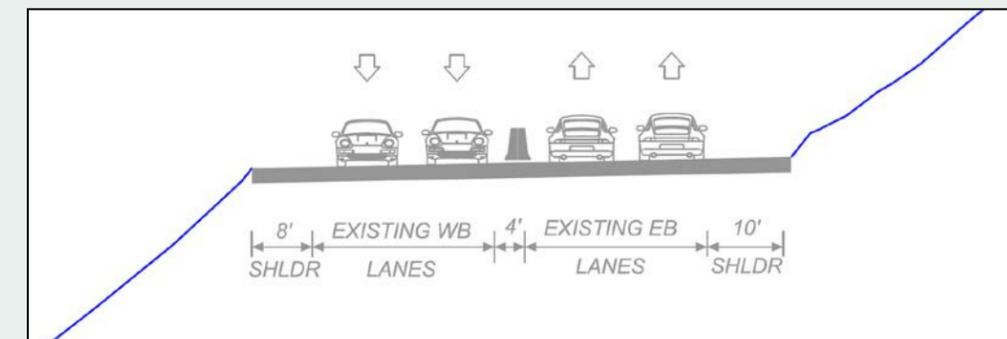
**Figure 14: Typical Section of Existing Conditions Section 1 – East of Wyomissing Boulevard Interchange**
