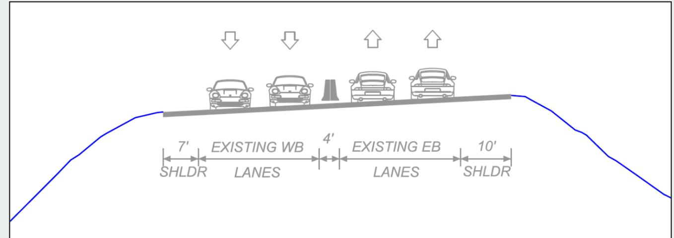
**Figure 18: Typical Section of Existing Conditions Section 2 – Penn Street Interchange to Lancaster Avenue**
