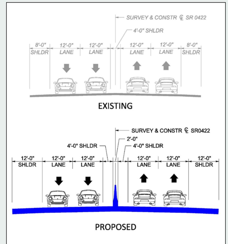
Figure 27: Existing and Proposed Typical Section for Four Lane Section
